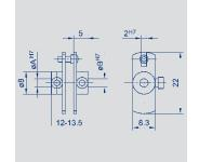
Fork coupling for 4 mm shaft diameters, low backlash
